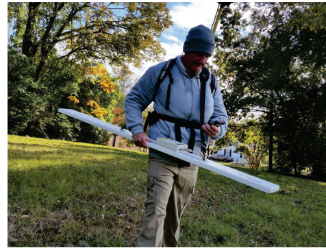
Electromagnetic instruments: GEM-2 (left) EM-61 (right)
